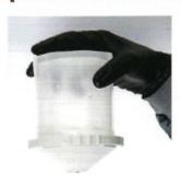
Competitor A's vented hard cup system dispensed all fluid in the cup but produced a major restriction and an inconsistent "glugging" paint flow.
