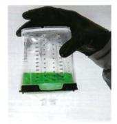
Competitor B's liner system created a major restriction in the liner, showing that it would starve the spray gun of fluid and create inconsistent flow. The final 8 oz. of fluid in the cup would not flow out
